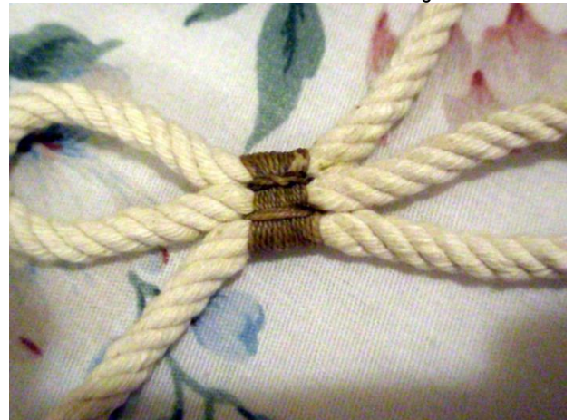
Correct placement and working of seizing
