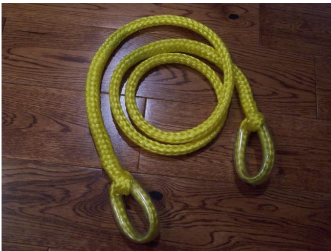
Completed hitched and tucked rope ends
