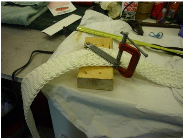
Cutting the sennits at a 45 degree angle using a hot knife
