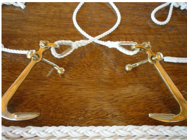
The brass items were tied together using 1/4 inch 3-strand nylon cord with eye splices at the ends
