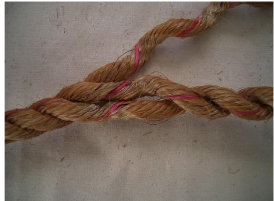
Lay-up first strand, skipping one turn.
