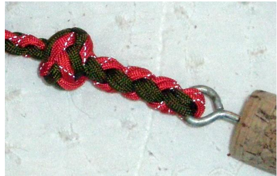
Becket Splice for 4-strand Square Sennit
