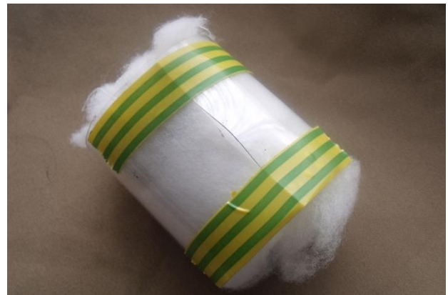
Mandrel with stuffed cavity
