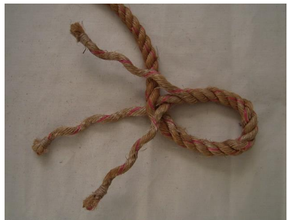
Place first tuck in "relaxed area". Continue in usual fashion to complete splice.
