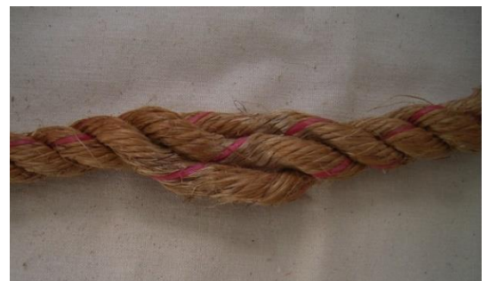
Lay-up next strand leaving room to tuck. Re-lay all strands as far as required.
