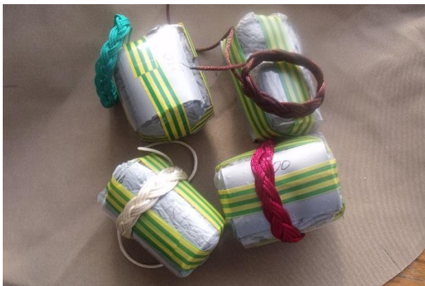
Mandrels in use – making various sized Turk's Heads
