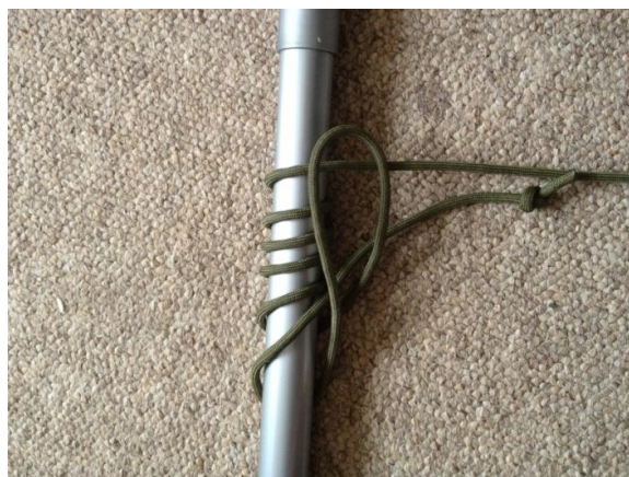
Pull the loop around and capture the working end
