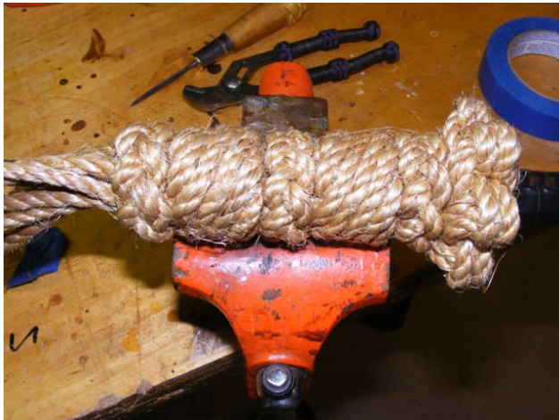
Fig. 6 – Add another Matthew Walker Knot and a single pass Diamond Knot.
