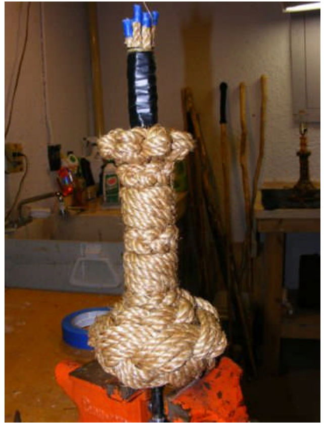
Fig. 9 – Next, tie a four pass Diamond Knot and carefully work it into a globe shape. This step can be frustrating. The bitter ends can then be tucked up into the inside of the knot or trimmed off once you have the desired shape.
