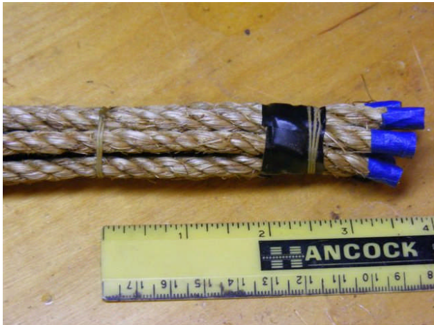
Fig. 1 – Start with a 14 inch length of 1/8 inch pipe threaded on one end and, using Constrictor Knots, seize seven 6 foot lengths of 1/4 inch manila line, for a distance of 2 ½ inches to the threaded end.
