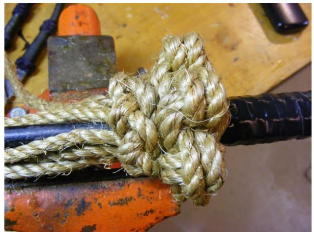
Fig. 4 – Next, tie a single pass Diamond Knot and work it tight.
