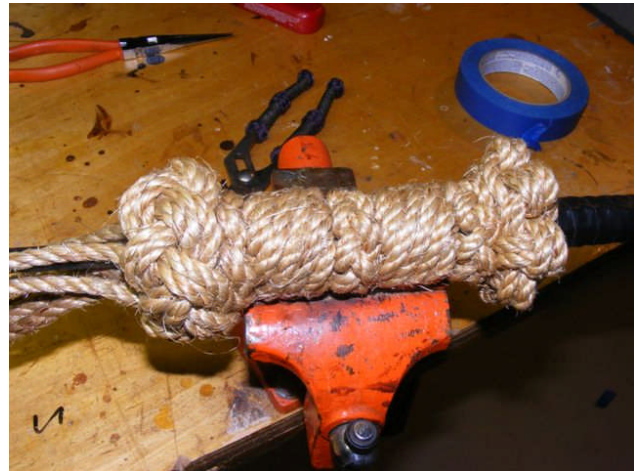
Fig. 8 – The finished two pass Diamond Knot.
