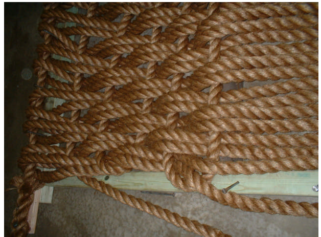
Weaving the strands over two under two.
