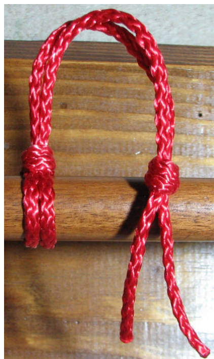
Finished with the Matthew Walker Knot
