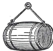
Fig. 6. Cask Slung with Can Hooks.
