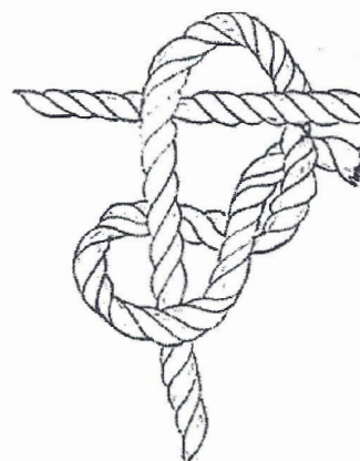
Method of attaching pendant cord to foundation cord.
